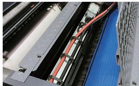
Inter-deck LED-UV curing unit over the impression cylinder
