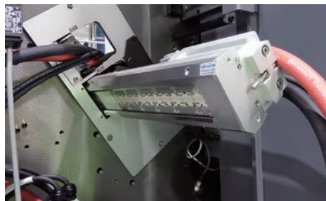
LED-UV curing unit in the delivery section
