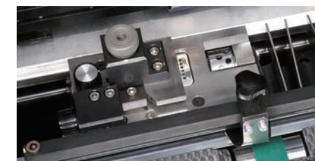
Pneumatic side lay device
