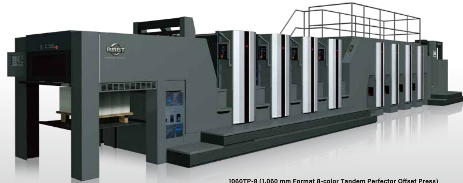
1060TP-8 (1,060 mm Format 8-color Tandem Perfector Offset Press)
